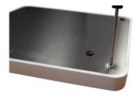
For mounting the reader, remove the cover from all feet and remove the screws (T15 Torx). The screw holes can be used to drill assembly holes (diameter  $\leq$  5 mm) and fixing the SIR-9151-UE with longer screws on a wall or below the table.
