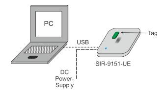
Since the reader is preconfigured for stand alone mode, after connecting SIR-9151-UE like shown above it starts reading UHF transponders. Recognized EPC Codes are transferred via the USB interface and can be received on a PC, e. g. using a simple terminal program.
